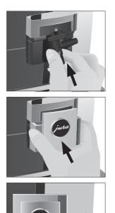
► Fit the assembled individual parts back in the dual spout and press it firmly.
